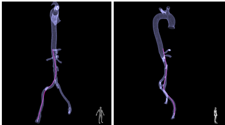
Visualization of a fiber optic shape sensor in an anatomical model.
